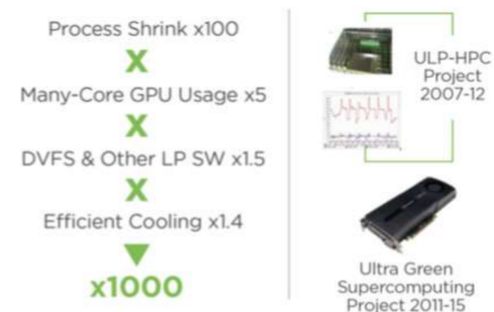
Fig. 1. The breakdown of 1000 times improvement in power efficiency in the ULPHPC project
