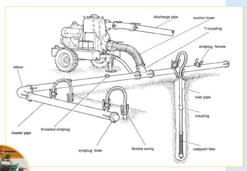
Wellpoint systems are broadly used and recognized in the construction of drainage systems for building trenches and excavations.
