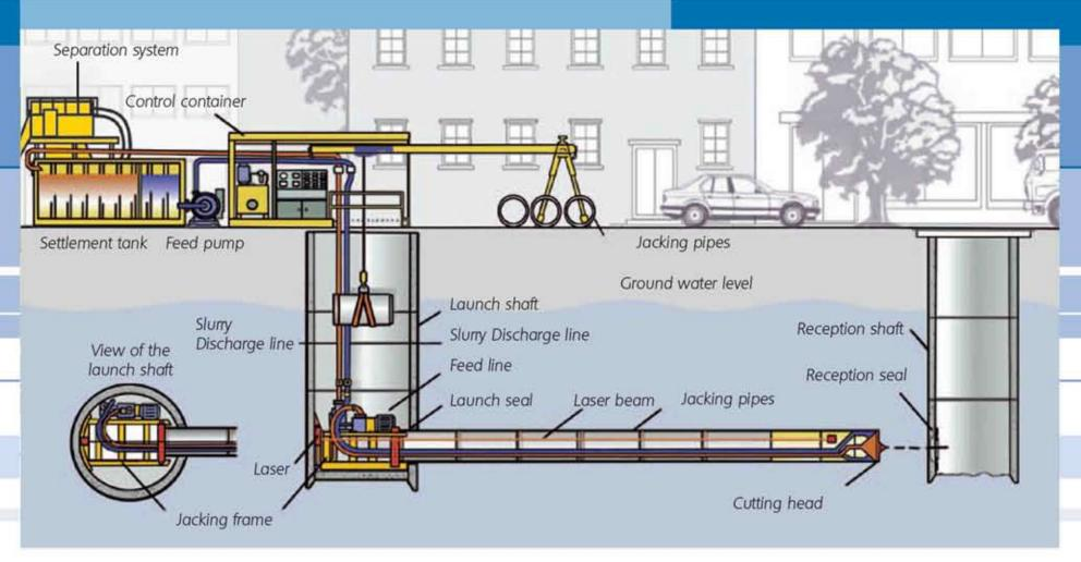
The cutter head (1) removes with its tools (cutters, knives, chisels or discs) the surrounding soil. This is taken to eh crusher chamber (2). This is where any stones are crushed (3).
